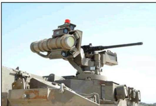
A high energy laser mounted on a remote weapons station
